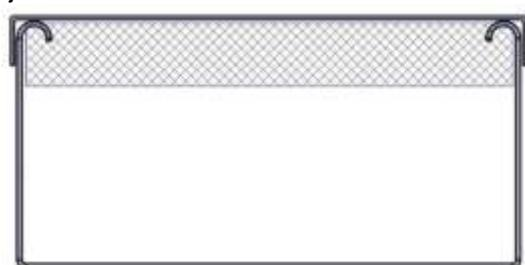
*The cable carrier volume depends on the height and width of the cable tray. When selecting the cable tray, it is necessary to provide for a volume reserve for possible subsequent installations of at least 30%.*
