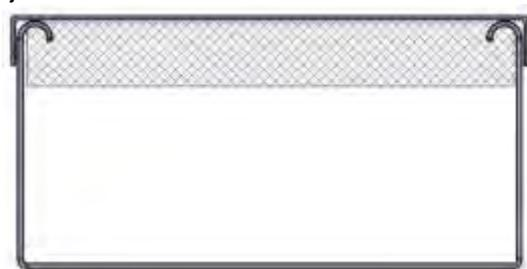
*The cable carrier volume depends on the height and width of the cable tray. When selecting the cable tray, it is necessary to provide for a volume reserve for possible subsequent installations of at least 30%.*
